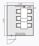
★Items 1 System wall 2 Company name plate 3 Fluorescent lamp 4 Electrical outlet (two-socket outlet x 1) 100V 900W or Energy saving pack 100V 400W 5 Electrical power supply
